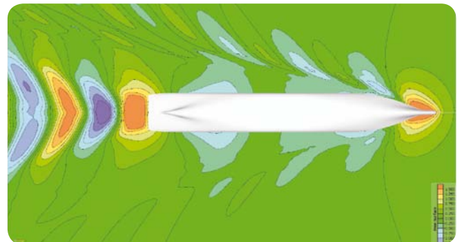
[Fig. 1] Optimization: baseline (upper half) vs. optimized hull (lower half) at design speed
