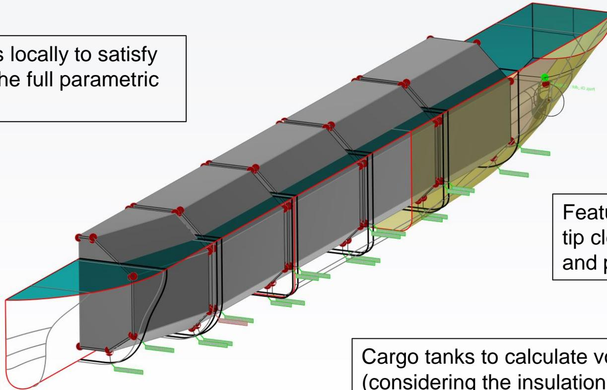
Realistic way of modeling twin-skeg stern (asymmetry between inner and outer skeg surfaces)
