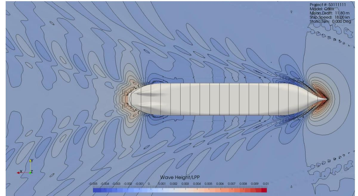
Optimization has NOT been carried out, but its estimated effective power is within 3-4% of a 210,000 m<sup>3</sup> hulls that had been built.
