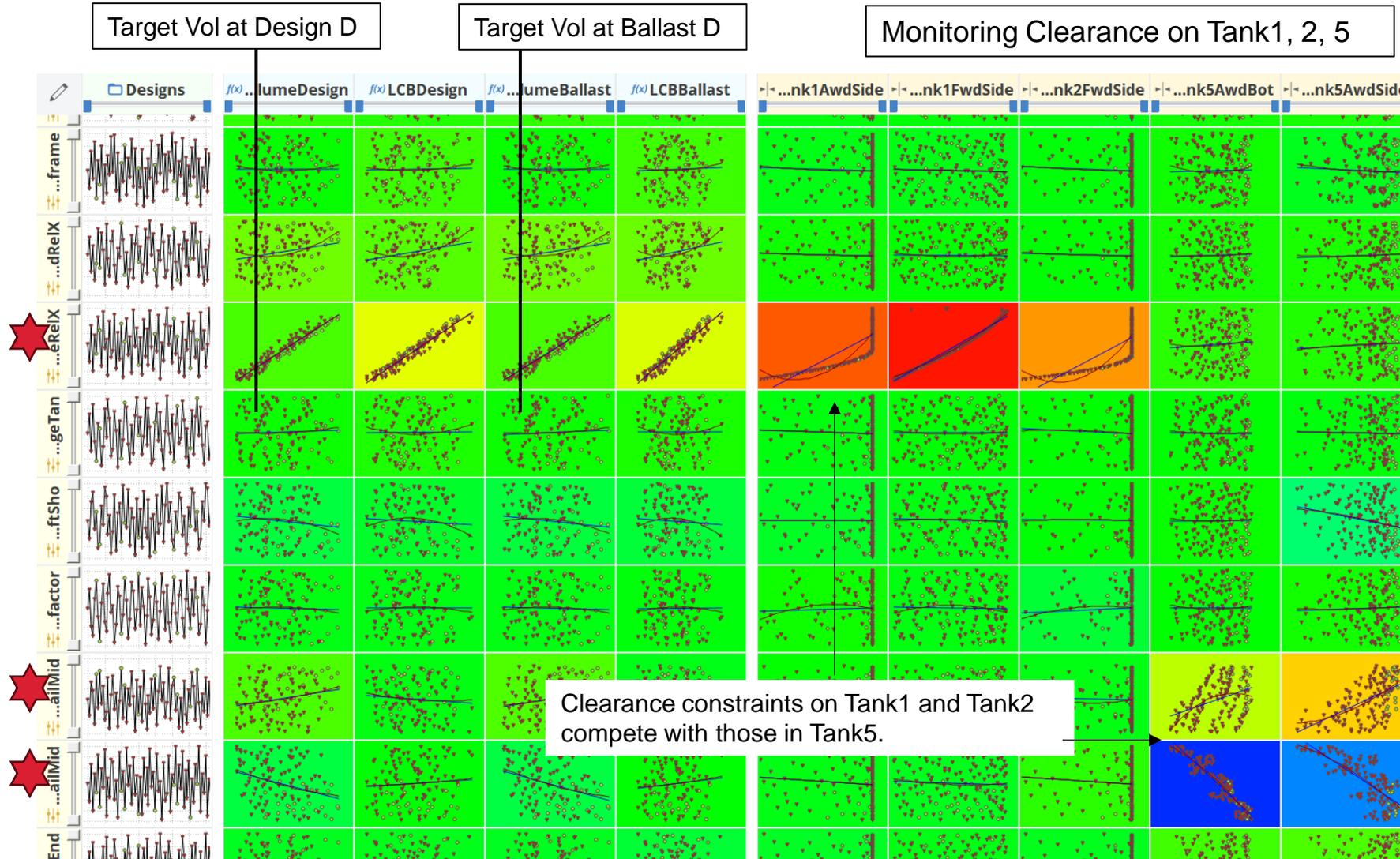
In this example, L, B, D and Tank Details (Size, Starting point, Cofferdam) are fixed. Also, a target displacement at design draft and ballast draft are known.
